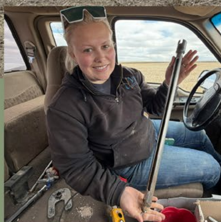
Here's the probe that gets pushed into the soil to grab a sample.
